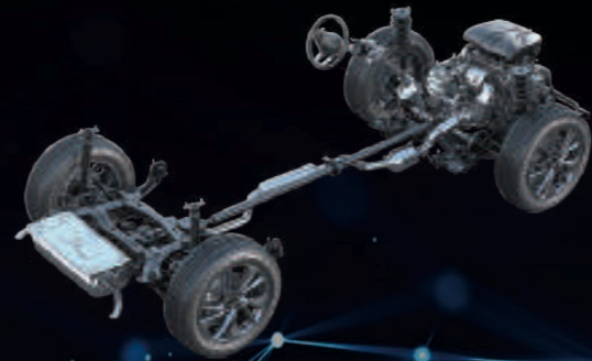
▶ Front Macpherson rear multi-link independent suspension + AWD
