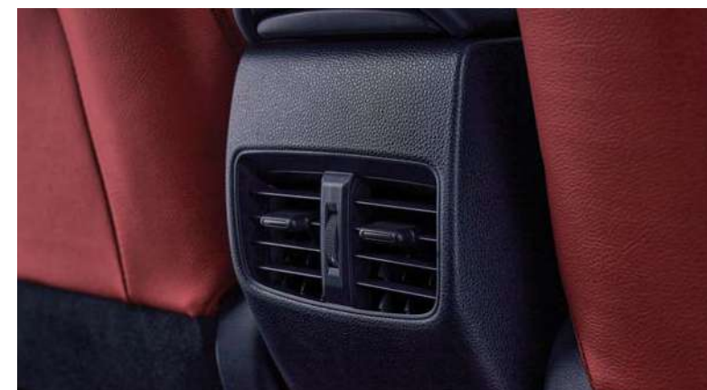
Rear Vents are located at the rear cabin to provide comfort to the passengers at the back.
