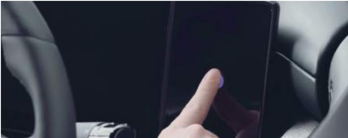
Remote Engine Start Fingerprint (AVN Authentication + Engine Start)
