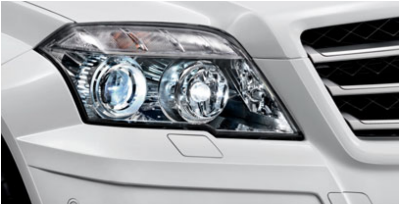
The Intelligent Light System with bi-xenon headlamps
