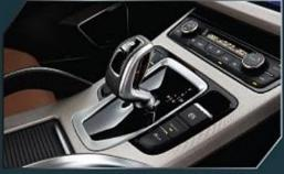
7-Speed Dual Clutch Transmission with Manual Mode
