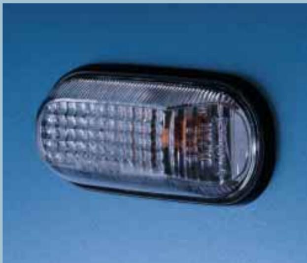
The indicator repeaters are located high on the side of the Honda S2000 for maximum visibility and are neutral in colour, to blend with the car's smooth lines.
